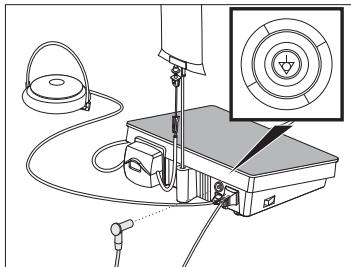
Clean the touch keyboard with a soft cloth with low fiber-release and position the sterile protective foil on the surface of the clean touch keyboard.
