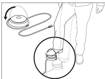
**PLEASE NOTE** The foot pedal comes equipped with a bracket that allows it to be moved to the place most suitable for the operation, without the need to use your hands to move it;
