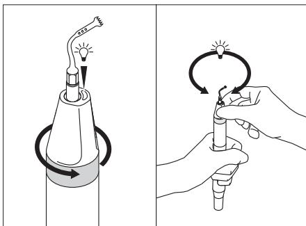
The position of the LED light on the front terminal of the handpiece can be adjusted in the following way:
