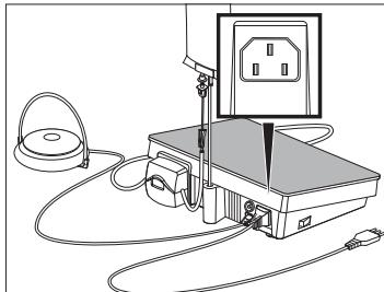
Equipotential plug: The device is equipped with an additional equipotential plug located on the rear of the console. This plug is in accordance with DIN 42801. Insert the connector of the equipotential cord (optional) to the plug on the rear of the device's console. The purpose of additional potential equalization is to reduce differences of potential which can occur during operation between the device's body and conductive parts of other objects within the medical environment;
