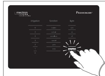
While the PUMP/CLEAN wording is flashing, press the foot pedal once and release it; the PUMP/CLEAN stops flashing and the irrigation circuit starts to fill up;
